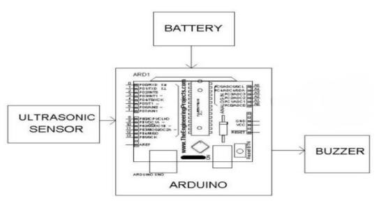
The Smart Blind Man Stick is an assistive device designed for visually impaired individuals. This project leverages the capabilities of the Arduino Uno microcontroller to develop a smart walking stick equipped with sensors that help the user detect obstacles, identify distances, and alert them using haptic feedback or sound. It aims to provide an enhanced experience for blind people by offering more safety and mobility
